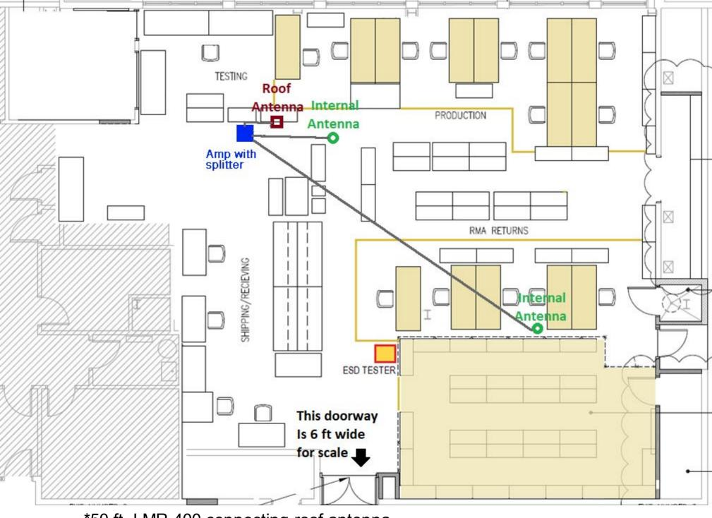
\*50 ft. LMR-400 connecting roof antenna and amplifier
