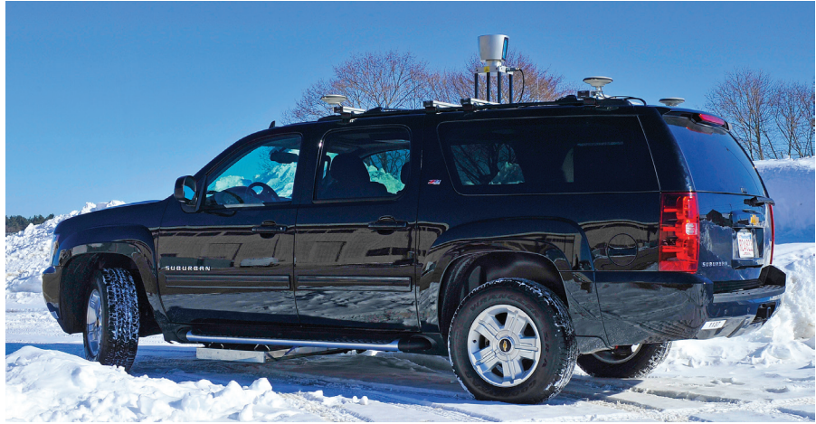
The Autonomous Systems Mobile Testbed vehicle has the waterproof localizing ground-penetrating radar array mounted underneath. Additional sensors, such as lidar, camera, and GPS/INS units, are used for verification and studying sensor fusion.
