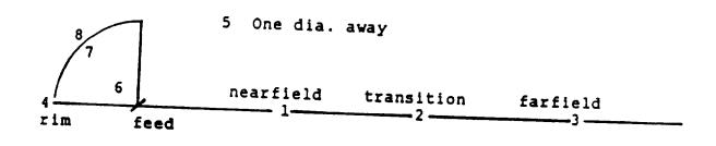
COMTECH OFFSAT ANTENNA VERTICAL PLANE RADIATION HAZARD LOCATIONS Horizontal line indicates main beam direction
