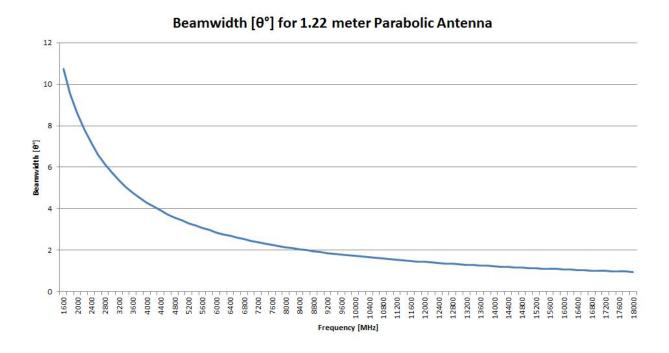
Figure 1: Beamwidth as a function of frequency [MHz]
