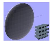
A schematic of a 6" lens antenna with 16 feed antenna array. The beams have an approximate beamwidth of 4.5 degrees and we are currently using WR-28 waveguide feeds as feed antennas.
