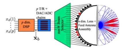
A schematic of the beamspace MIMO (multiple input multiple output) transceiver that uses a lens antenna and a feed antenna array for beamforming. This will serve as a transmitter and/or receiver in our experimental system.
