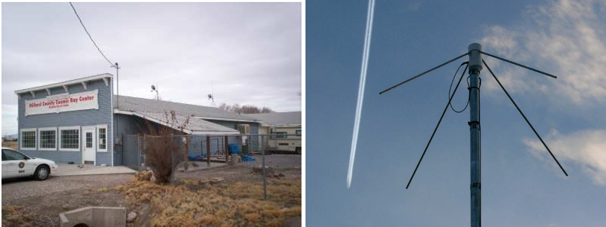
Figure 6: Left: The Millard County Cosmic Ray Center (CRC). Right: Homebrew crossed-dipole antenna tuned to 6 m (50 MHz) band, mounted on top of CRC for radio environment tests during summer 2009.
