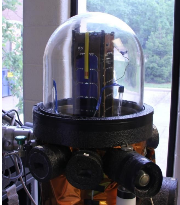
Figure 35: S3FL TVac Chamber testing the 3U CubeSat GRIFEX
