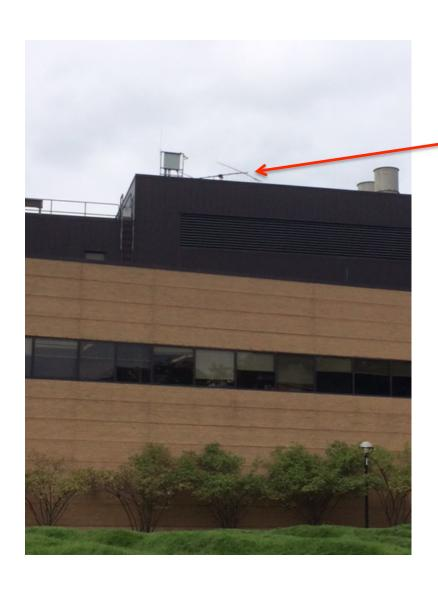
Note the antenna is direction And points to follow satellites. Gain is ~ 18 dBi.
