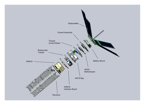
CADRE will test the Winds Ions Neutrals Composition suite (WINCS), developed by the Navy Research Laboratory. WINCS consists of four electrostatic analyzers and two mass spectrometers; it will measure the density, temperature and composition of the ionosphere. Four deployed solar panels and bus will fly in a dart configuration using a star tracker, IMUs, photodiodes and reaction wheels.
