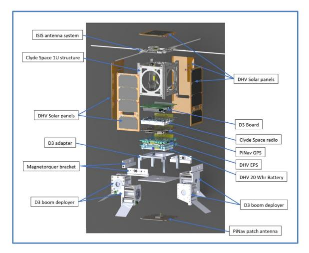
The D3 CubeSat is designed to test the D3 device, which enables a standard CubeSat for using the drag acceleration for orbital maneuvering. The mission will test a de-orbit point targeting algorithm developed at the University of Florida ADvanced Autonomous Multiple Spacecraft (ADAMUS) laboratory.
