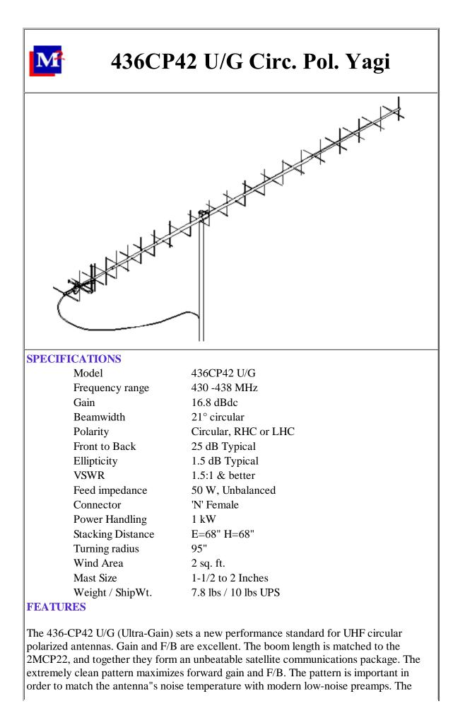
CP42 is also excellent for ATV, repeater operation, and long haul tropo DX and EME around 432 MHz.
