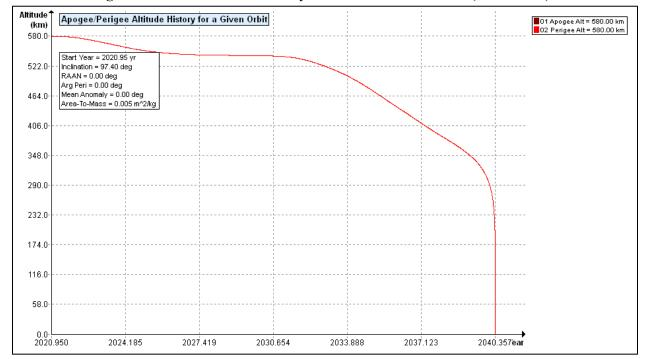
Figure 3. Worst Case Orbit Decay Profile for UMBRA SAR (DAS v3.0.1)
