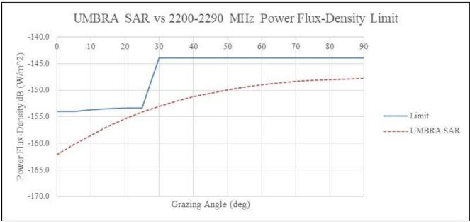
Figure 5. Power Flux Density for S-Band (2200-2290 MHz)
