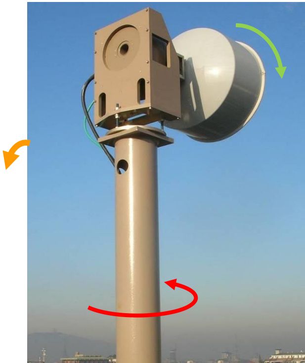
Fig.2: Outdoor test range: the AUT mount (left) and the upper SRC mount (right).
