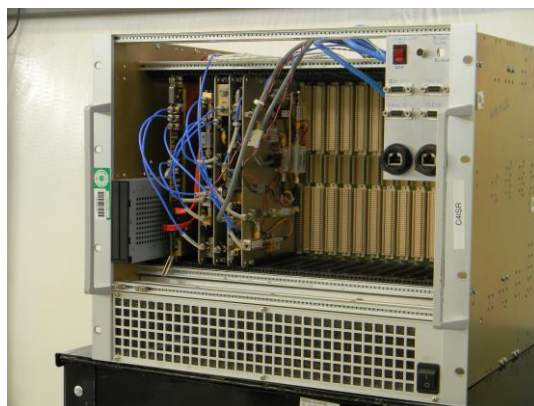
Figure 1. The FlexSAR-X VME chassis.
