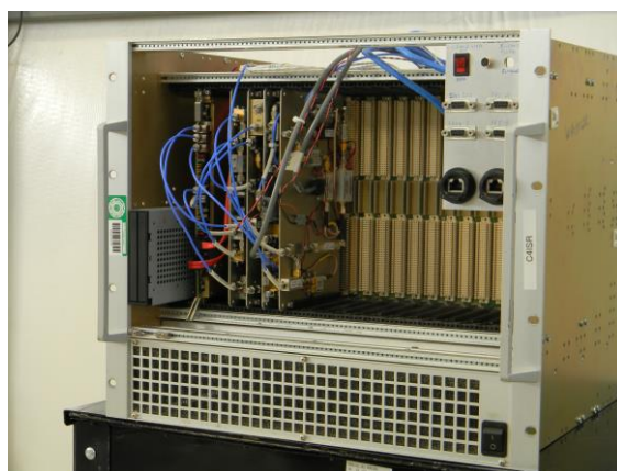
Figure 1. The FlexSAR-L VME chassis.
