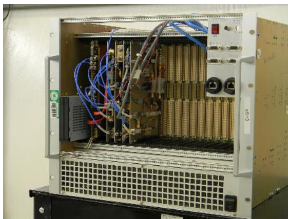
Figure 1. The FlexSAR-X VME chassis.
