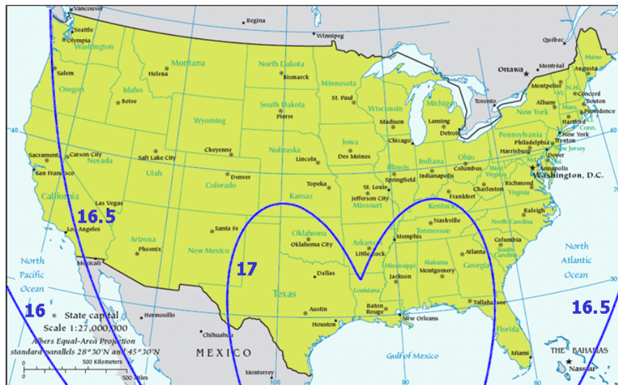
Figure 15. GSO-Plane Beamwidth and Maximum PSD at 14.25 GHz for ThinSat 300 Operating Tilted 10° Northward with a Satellite at 93° W
