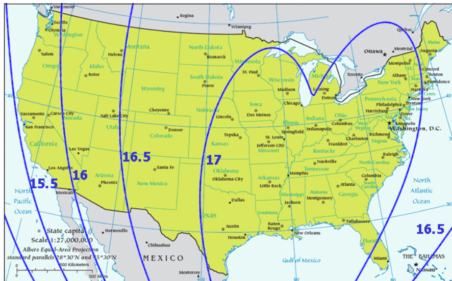
Figure 14. GSO-Plane Beamwidth and Maximum PSD at 14.25 GHz for ThinSat 300 Operating Tilted 10° Westward with a Satellite at 93° W
