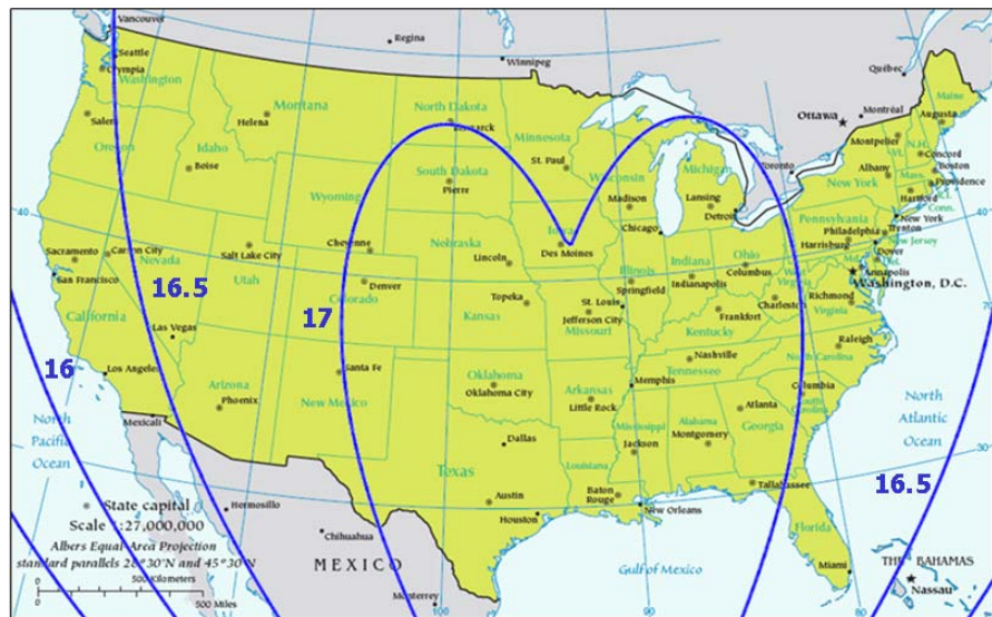
Figure 13: GSO Plane Beamwidth and Maximum Power Spectral Density at 14.25 GHz for ThinSat 300 Operating with Satellite at 93° W
