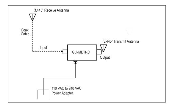
Figure 2. GLI-METRO System Block Diagram
