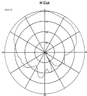
Figure 2-2. Far Field Plots Azimuth Cuts
