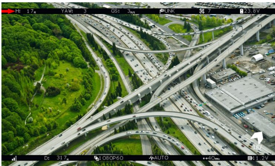
Figure 6. OSD View - With Additional Telemetry Information
