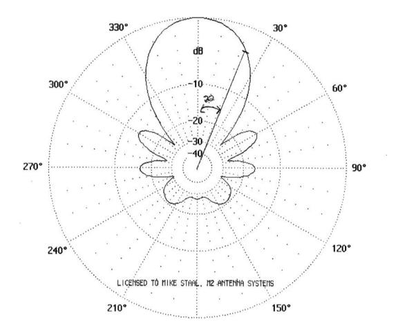
Station Configuration is Quad Yagi; above pattern is typical for each of the 4 Yagi antennas used.
