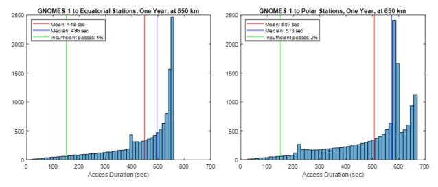
Figure 2.4-3. Pass lengths for GNOMES-1 at 650 km 37° inclined orbit (labeled "Equatorial") and 650 km sun-synchronous orbit (labeled "Polar").
