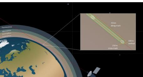
Figure 3.1-1. Dimensions of the occulting GNSS signal ray path
