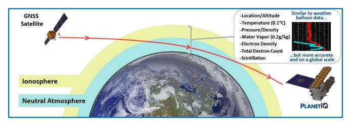
Figure 1.2-1. Geometry of a typical GNSS-RO event and resulting data products derived from the technique
