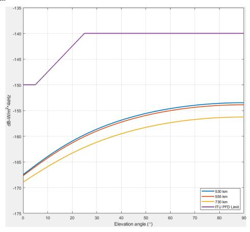
Figure 2.4-1. PFD at the Earth's surface produced by the X-band downlink radio for GNOMES-1 at all possible injection altitudes.
