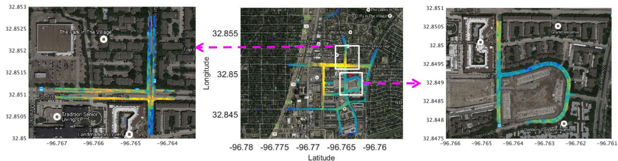
Figure 3: Minimum (left) and maximum (right) path loss exponent in a multi-family residential area.
