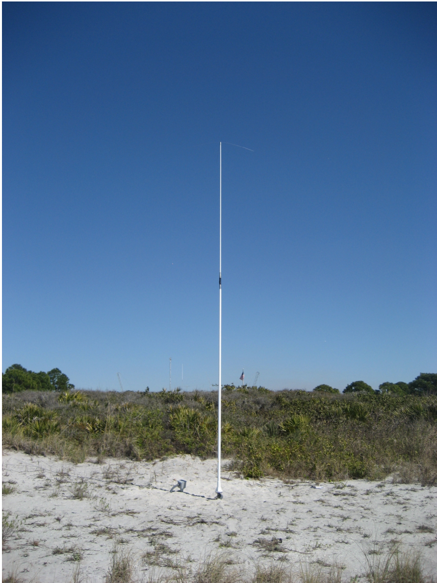
Example of CODAR Transmit Antenna
