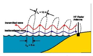
This over the horizon oceanography radar can pick up back-scattered signals (Bragg effect) from ranges of up to 200 km.
