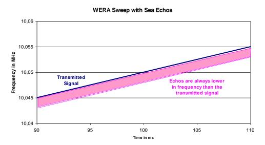
The receiver is continuously switched on, to pick up signals from all over the defined range. These systems provide best signal to noise performance due to the extreme low noise FMcw transmission mode.
