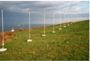
The WERA receive antenna array consists of 8 to 16 vertical mono-poles to build a linear array. Software beam forming is used to steer a beam over an angel of about +/- 60 degrees.
