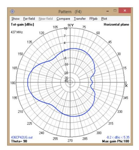
Transmit Power 18.7506 dBW 75 W Coupling Loss -3. dB Antenna Gain 14.2 dB RHCP EIRP 29.9506 dBW 988.693W Path Loss -154.8 dB 437 megahertz 3000 kilometers Antenna Gain 0. dB Average Polarization Loss -3.0103 dB Dipole Coupling Loss -0.11 dB  $1.59605 \times 10^{-13}$  W Received Power -127.97 dBW 1200.K Receiver temperature Bit Rate 9600.b/s Eb/NO 30.0151 Threshold GMSK Theoretical 10^-4 BER 9.4 dB Demod loss Practical -3. dB Link Margin 17.6151 dB
