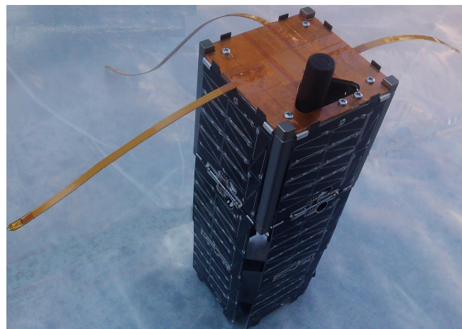
Figure 2: Satellite with deployed antennas and solar panels
