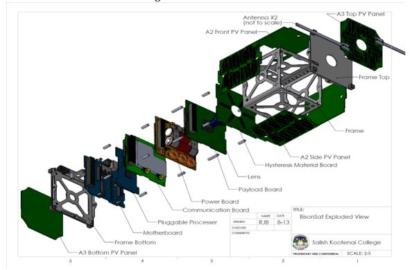
BisonSat has primarily an educational objective of training undergraduate engineering and science students on design, build, test, and operation of space hardware. The science payload is a visible light camera for land cover classification, and cloud cover and cloud height measurements.
