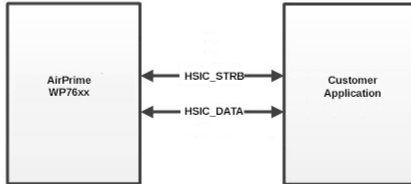
Figure 4-11: Example of 2-wire HSIC Bus Application
