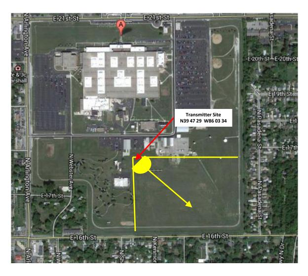
Test site is fenced, antenna is 9 meters above ground with 90 degree horizontal and 8 degree vertical scanning angles
