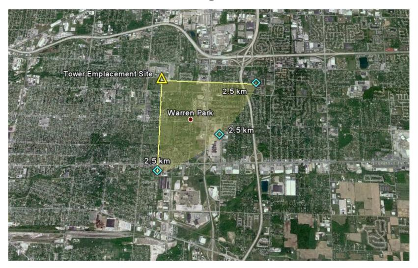
Range will be limited to 2.5 km during the short durations the radar is operational
