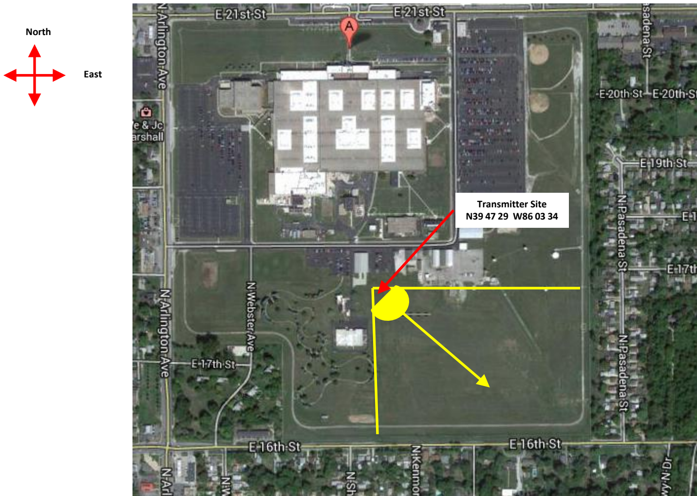
Test site is fenced, antenna is 9 meters above ground with 90 degree horizontal and 8 degree vertical scanning angles
