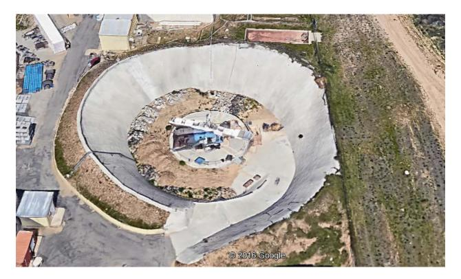
The Raytheon hardware will be positioned at one end of the beam in the center of the centrifuge. The other end will have a calibrated weight on it to counterbalance the Raytheon hardware when the centrifuge is in operations. All the testing is below the rim of the centrifuge.
