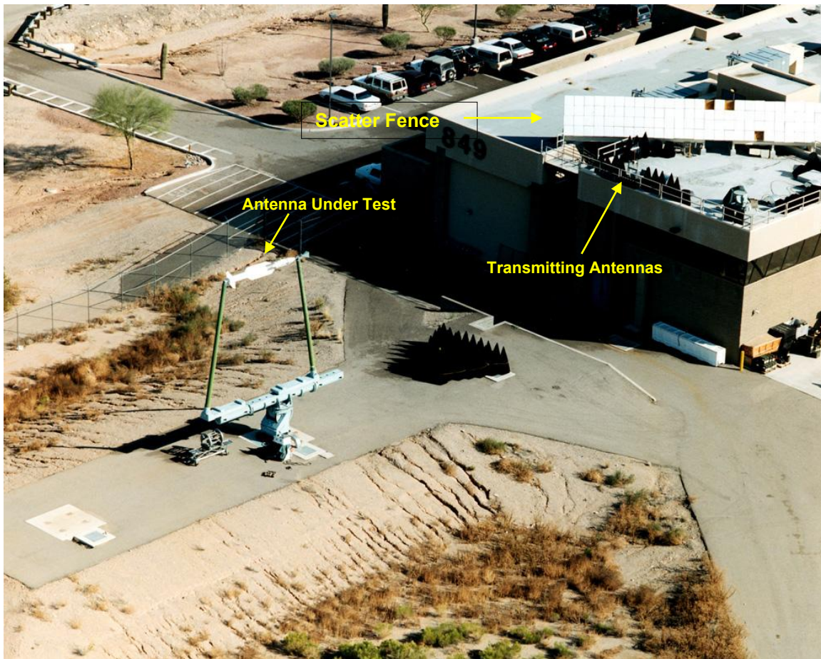
Antennas are directional with a very narrow beam, the transmitters point to the desert & sparsely populated Indian reservation land.
