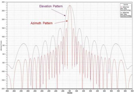
Figure 1 Anticipated Beamforming Antenna Pattern
