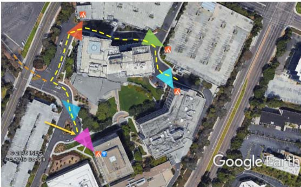
Figure 2 Directional Antenna Orientations
