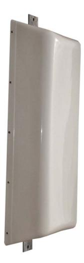
**Single bay** broadband four dipole panel covering the 470-700 MHz spectrum. The radiating elements and structural dipoles are entirely welded to the support spine. This results in an enhanced reduction in PIM, even after many years of being in service.
