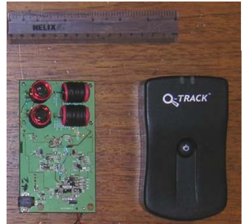
Q-Track QT™-400 tag transmitter prototype with four element antenna array.
