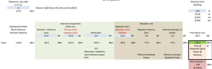
Effective Radiated Power (W) 100 feet from the building 1.99526E-11 in Watts Same in pico Watts 100 feet from the building 19.9526231496888 pW
