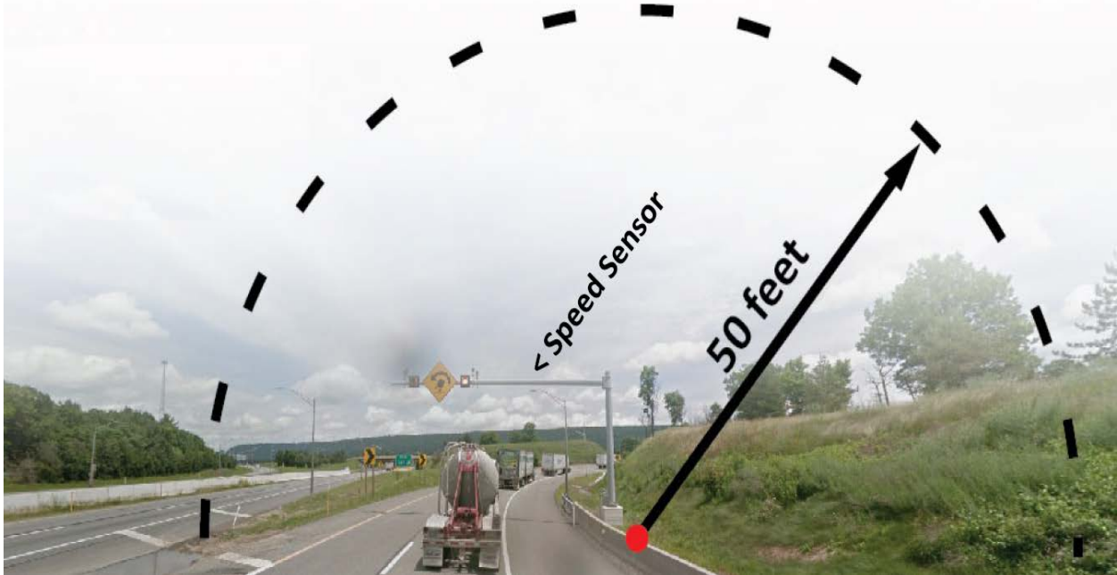
Figure 3 - Radiolert Transmission Distance
