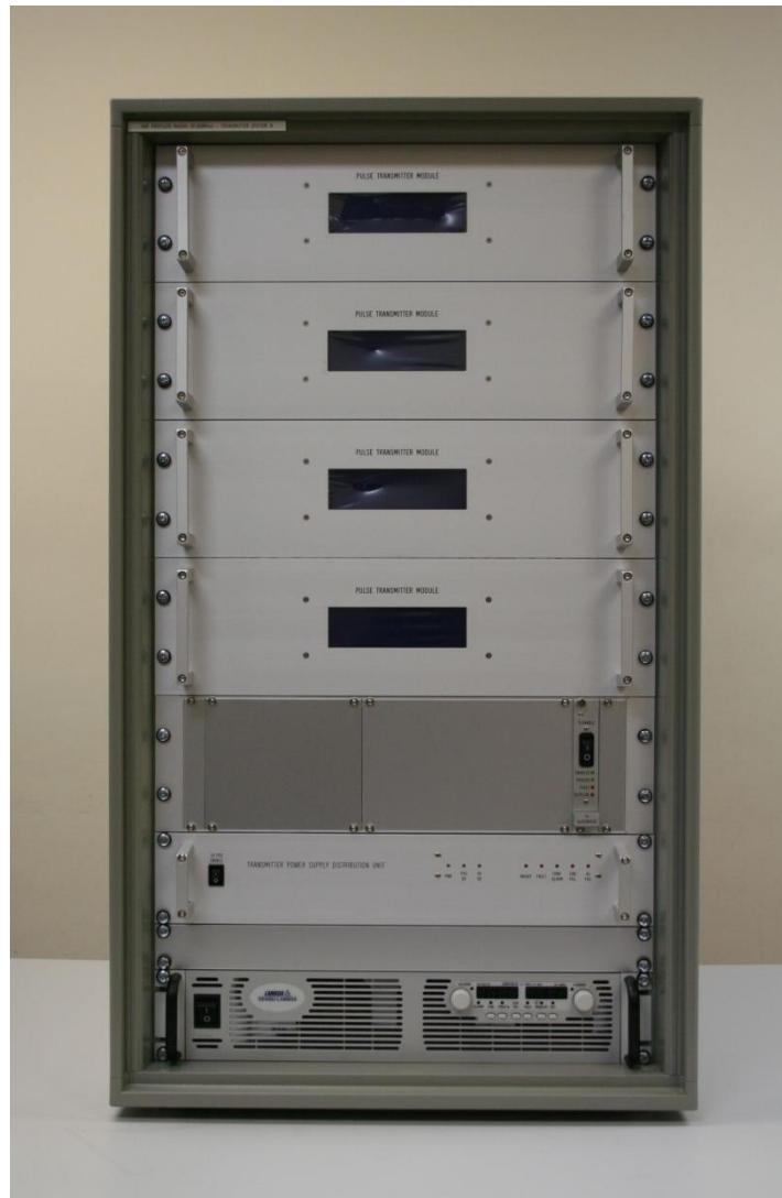
Pulse Transmitter System Comprised of Four Pulse Transmitter Modules
