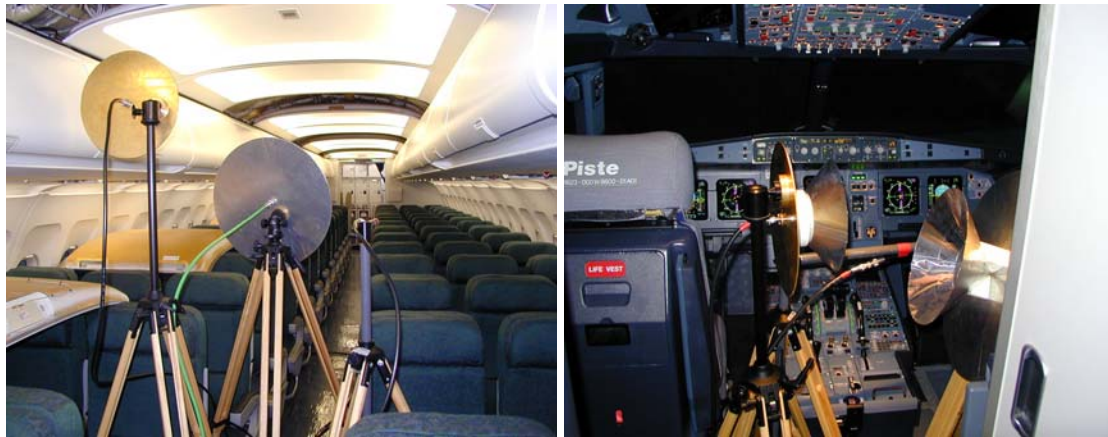
FIGURE 27 - ANTENNA SET-UPS FOR CABIN AND COCKPIT TESTS
