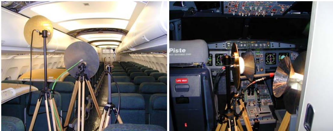
FIGURE 27 - ANTENNA SET-UPS FOR CABIN AND COCKPIT TESTS
