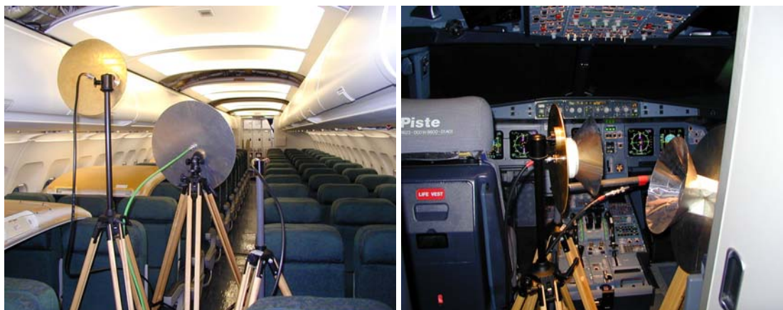
FIGURE 27 - ANTENNA SET-UPS FOR CABIN AND COCKPIT TESTS
