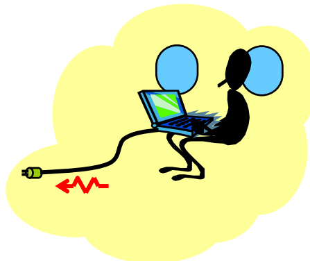
FIGURE 3 : CONDUCTED COUPLING TO AIRCRAFT WIRING
