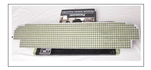
The Ku-band Antenna is designed to receive and transmit commercial Ku-band satellite signals consistent with the FCC's earth stations aboard aircraft (ESAA) rule. See 47 C.F.R. §25.227. The antenna is interconnected to a broadband controller; satellite modem, power supply and ARINC 429 bus.
