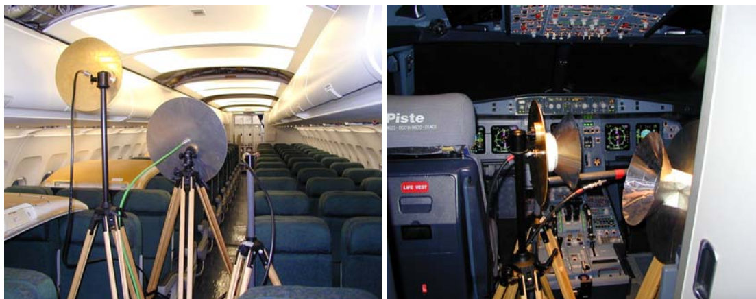
FIGURE 27 - ANTENNA SET-UPS FOR CABIN AND COCKPIT TESTS
