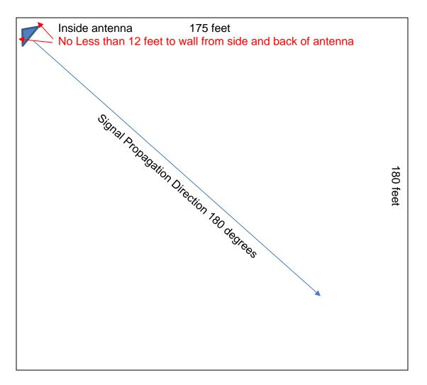
Directional antenna transmits signal towards opposite corner. Signal outside hangar at 100 feet: less than -140dBm.
