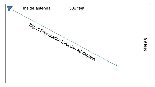
Directional antenna transmits signal towards opposite corner. Signal outside hangar at 100 feet: less than -145dBm.
