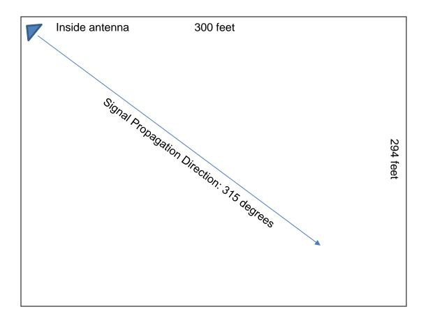
Directional antenna transmits signal towards opposite corner. Signal outside hangar at 100 feet: less than -145dBm.
